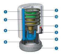
Emmeti have developed a new generation of Electrothermic heads, built around a sensitive wax/copper element, for responsive actuation. Includes pop up indicator to show the valve in the open position, for ease of installation and maintenance. The loose ring threaded mounting can be used one handed, and the oval body shape allows finger space between each head.
