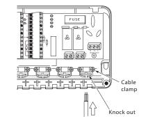
It is suggested to use the the turretts for the smaller actuator cables, and the cable entries or rectangular knock out points for the mains cable, room thermostat cables and cables to the boiler and pump.
