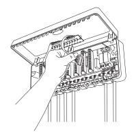
Rotate the cover down and close, securing with the 3 screws on the bottom of the cover.
